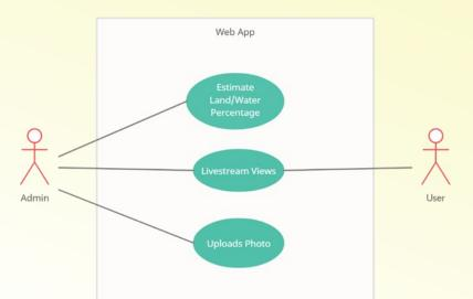
The figure above depicts the architectural diagram of web app. The admin checks if the area in the image is filled with water or not. The user will be capable of performing the following tasks:
